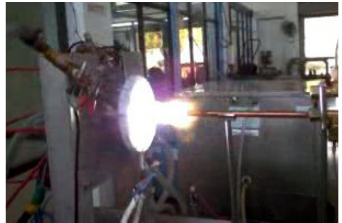
Figure B.1.1.2 : Photograph of the torch in operation along with enthalpy probe
