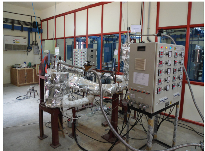
Figure 2.3.2 Pump driven Lead-Lithium loop at IPR
