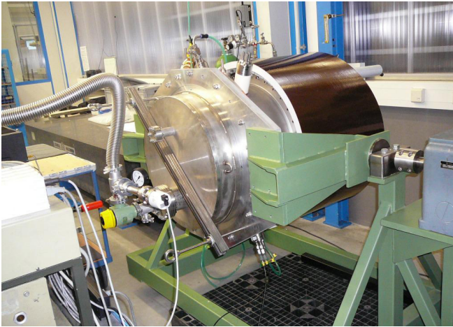
Figure A.2.4.1. Acceptance test of the accelerator system for ROBIN ion source at M/s PVA, Tepla, Germany
